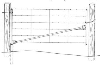
The bolted joints between the diagonal and the ends must be tight to hold the latch end vertical. McRae welds tabs of sheet steel (5/16" or 3/8" stock) 2-3 inches square to the gate ends and bolts the diagonal to these. (Figure 2). Bolted joints let you adjust the angle of the diagonal if the gate sags or rides too high but don't let the latch end lean "in" or "out". If the gate is hinged on the lower side, you can adjust it to close at the right height even on sloping ground. The ends of the
