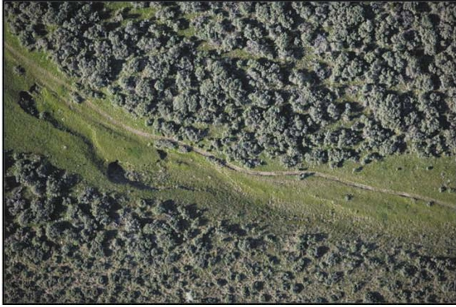
Figure 9. Multiple headcuts in what was once a stringer meadow. Image acquired 100 m above ground level from a light sport airplane at ~20-mm per pixel resolution.
