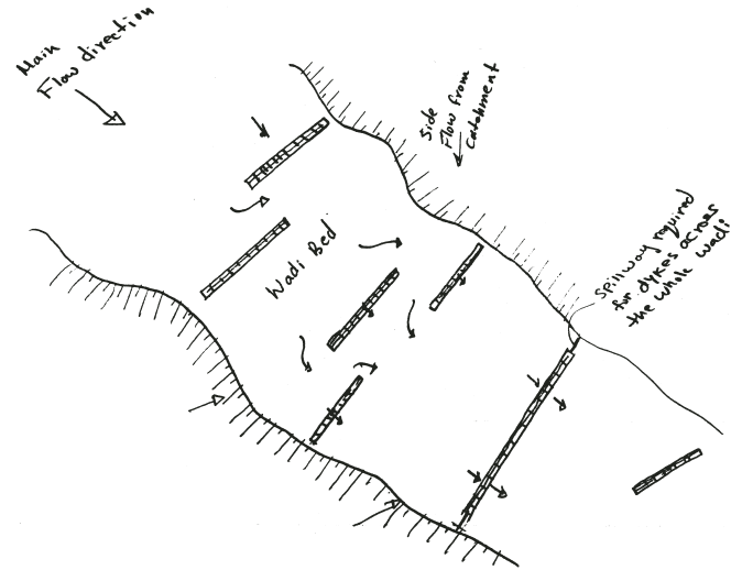
Figure 1a. Schematic of stone dykes to maximize infiltration of water into wadi channels.
