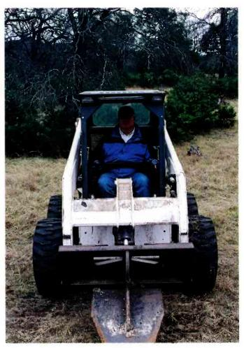
**Figure 2.** Royce Pyssen driving the skid-loader with the grubbing attachment.
