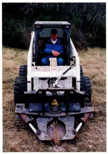
**Figure 1.** Royce Pyssen, Allison's dad, driving the skid-loader with the hydraulic shearing attachment.
