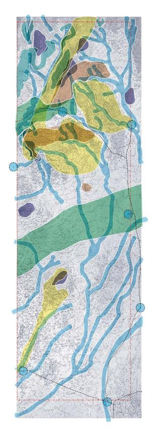
**Figure 3.** If part of the ranch is going to be developed or subdivided, mapping of resources should be used to plan building sites, lot lines, and roads for minimum impact on things like waterways, view shed, and wild-life habitat.
