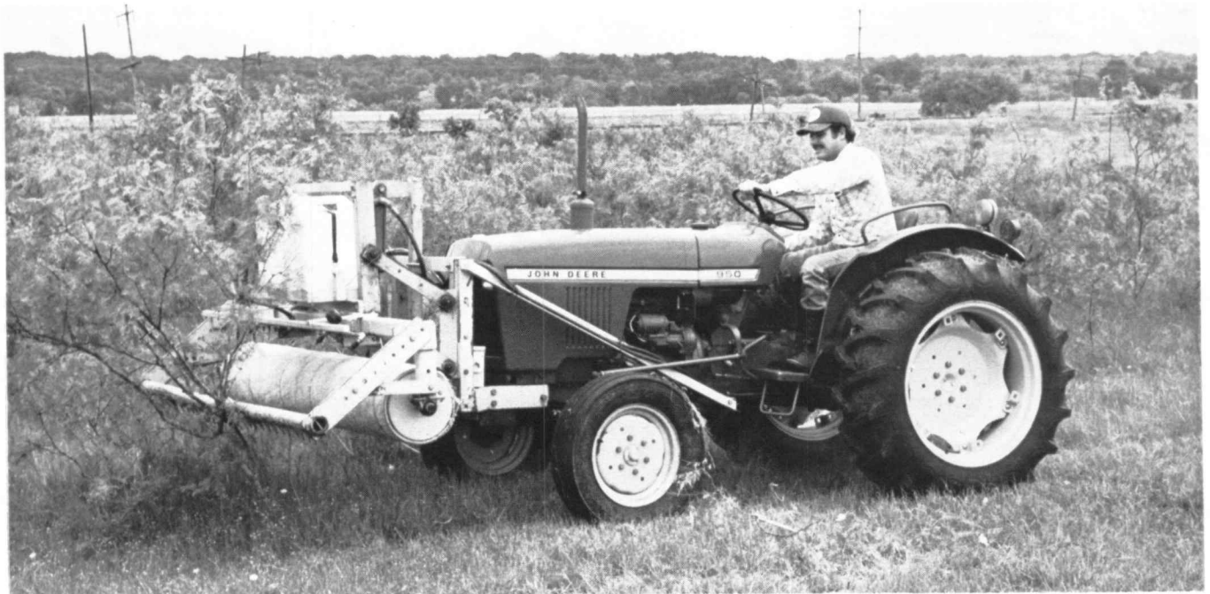
A herbicide solution is applied to small honey mesquite trees with the carpeted surface of the rotating cylinder mounted in front of the tractor.
