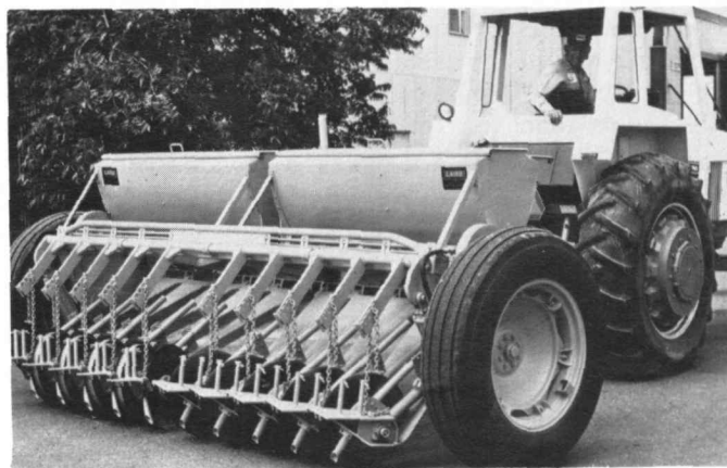
Hydraulically operated opener arms lift attachment for Rangeland Drill. Down.
