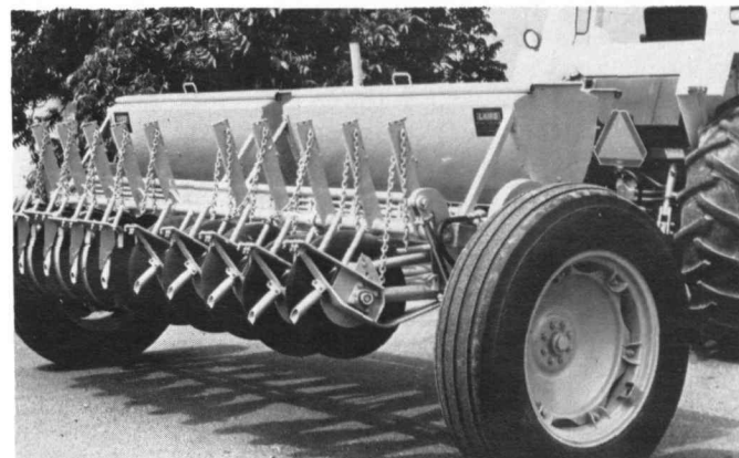
Forest Service Hydraulically operated opener arms lift attachment for Rangeland Drill. Up.
