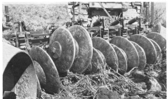
Sungeneral of Australian stump-jump plow. Note raised pair of disk.
