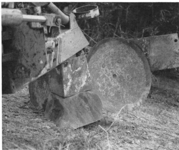
Sieco fireflow that makes a scalp 30 inches wide and 9 inches deep.
