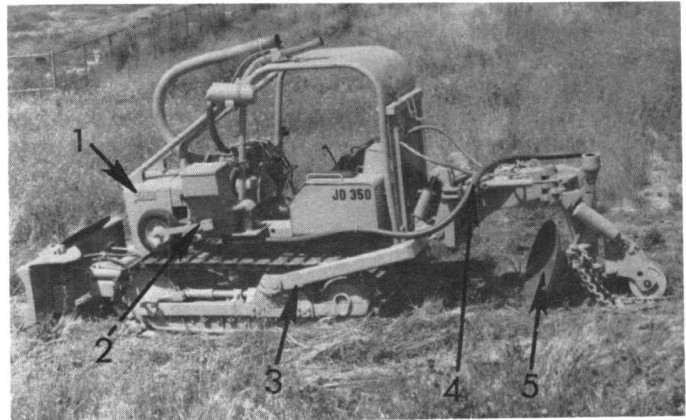
Five component interseeder: (1) prime mover, (2) seed-metering device (thimble seeder), (3) implement-carrying hitch, (4) seed-transfer system, and (5) scalper.
