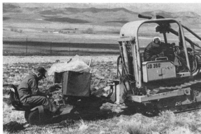
Workers transplant a variety of shrubs with a modified Whitfield tree transplanter equipped with a v-shaped, double-sulky type scalper.
