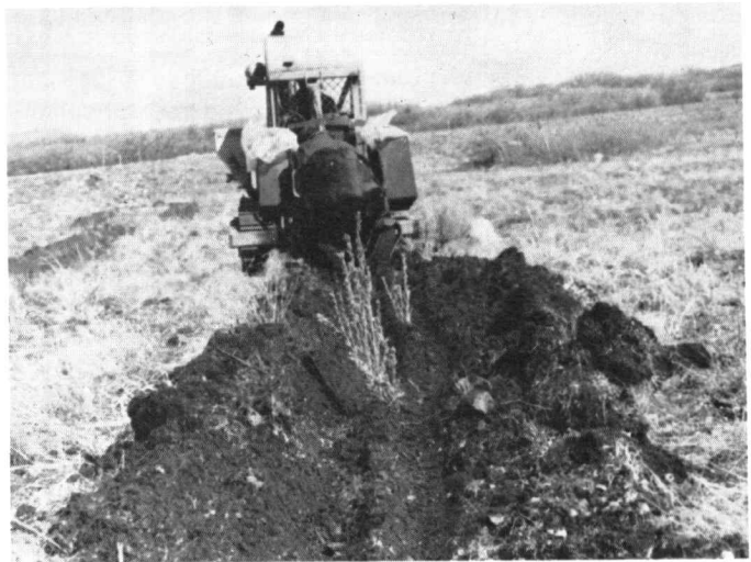
Mountain big sagebrush, transplanted with the modified Whitfield tree transplanter, obtained an 80% survival success rate after 2 years.
