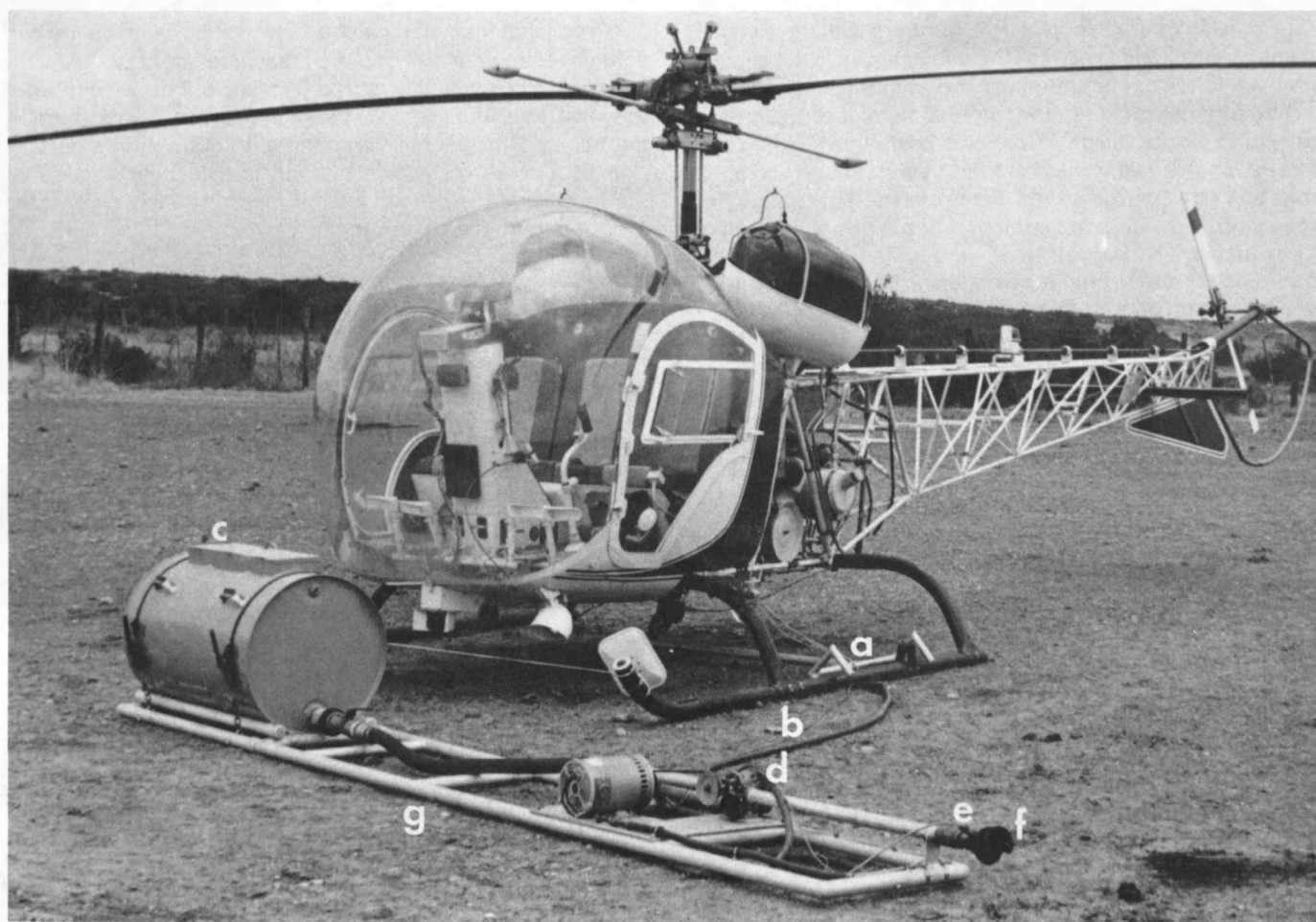
Fig. 1. Helitorch is composed of a spreader bar (a), electric power cable (b), fuel drum (c), fuel pump (d), ignitor (e), nozzle (f), and support frame (g).
