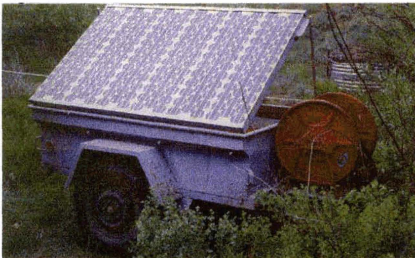
Trailer set up near Sawtooth Creek. Six 33-watt panels provided 198 watts of 12 volt power.
