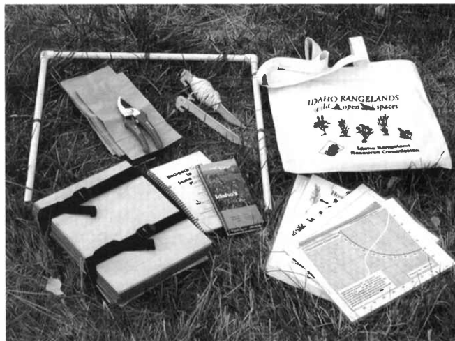
Figure 3. Contents of the range assessment equipment kit.
