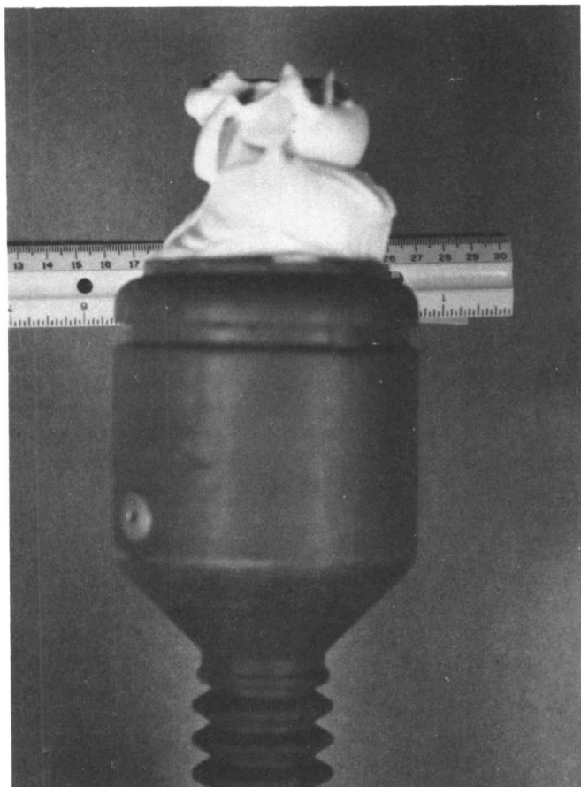
Foam emitter nozzle. These hang from end of boom. Enlarged tip accumulates a glob of foam which hangs on brush when it drops. Elongated neck of nozzle is flexible if boom drops into brush.
