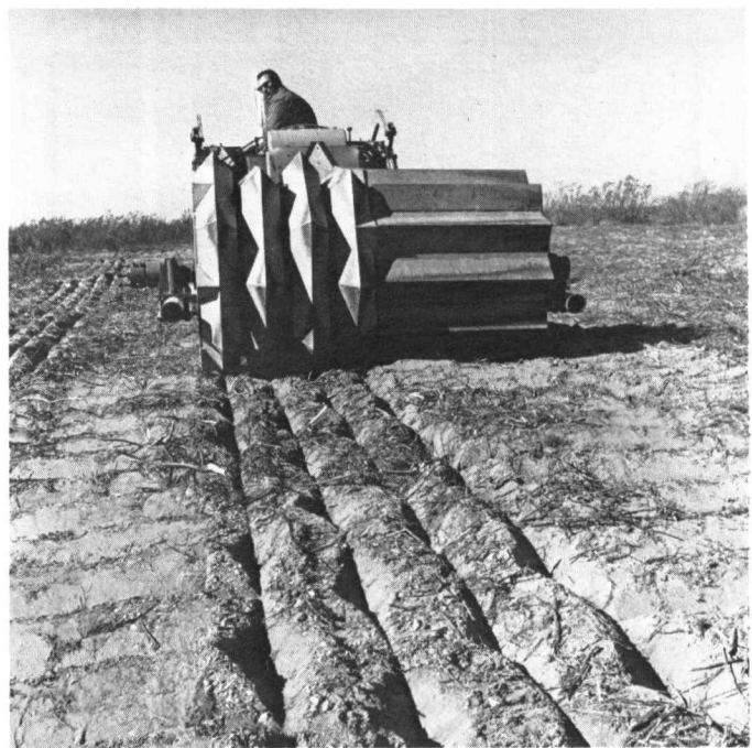
The land imprinter forms two sets of interconnected furrows with the downslope furrows shedding rainwater into the cross slope furrows, where it infiltrates deeply to germinate seeds and establishes seedlings.
