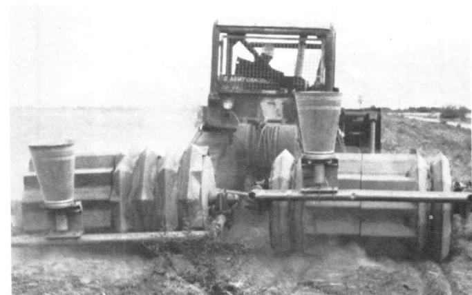
Two imprinters in tandem with broadcast seeders mounted. This operation is near Fort Huachuca in southern Arizona, where 500 acres of bull-dozer-cleared shrub-infested rangeland were seeded to weeping lovegrass in 1978.
