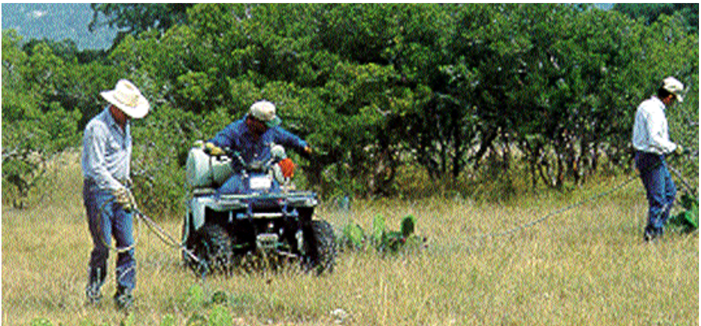
Fig. 1. ATVs make excellent spray platforms. This 4-wheel ATV, equipped with a 25-gal spray tank and 12-volt "Shurflo" pump, supports three spray guns, and covers a 40-ft-wide swath.
