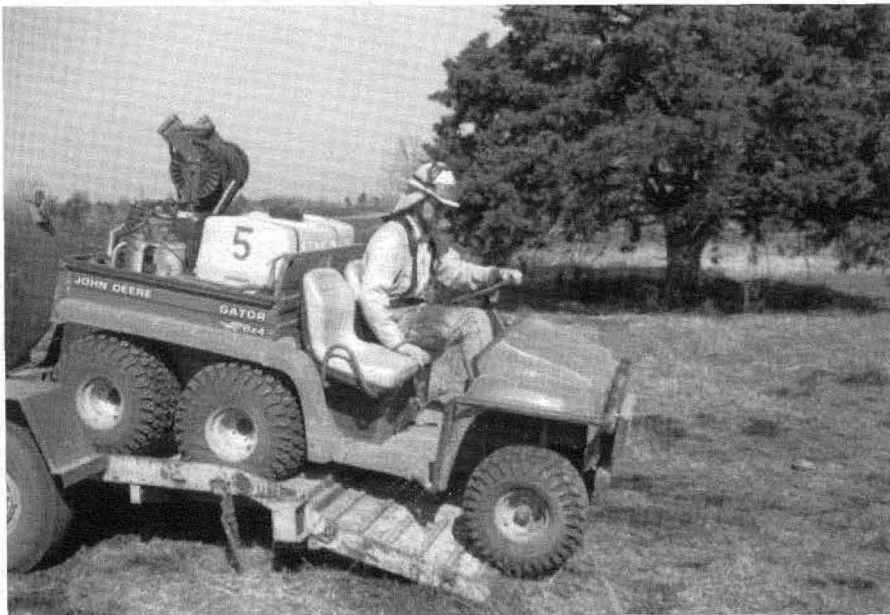
The Gator is outfitted to carry a slip-on pump unit for suppression needs and it also carries personnel, equipment and fuel on the fireline.
