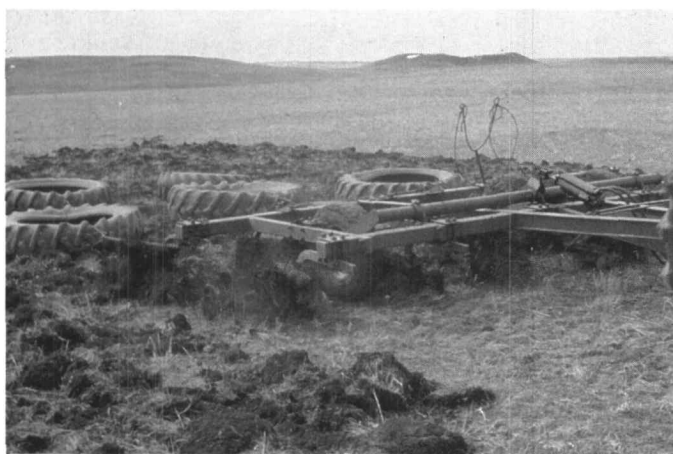
Fig. 5. Dragging tires behind the chisel plow did not increase clubmoss control.
