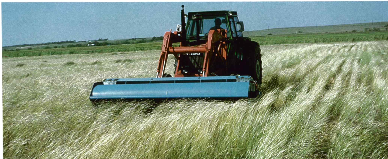
Harvesting 'WW-SPAR' Old World bluestem with the Woodward flail-vac seed stripper. ARS, Woodward, Okla.
