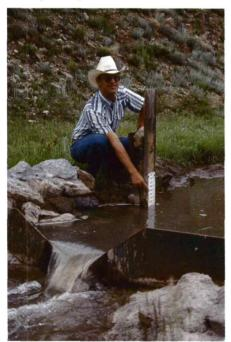
SCS District Conservationist Burl Boren checks stream flow at U.S. Geological Survey sediment check point on Badger Creek.
