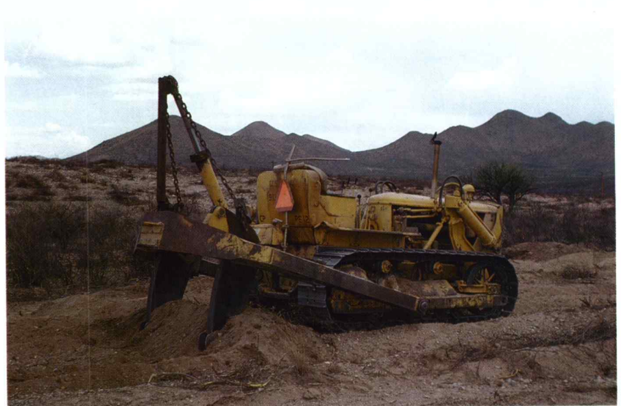
Fig. 5. Root-plow behind a bulldozer is an effective mechanical treatment for killing semiarid rangeland shrubs.
