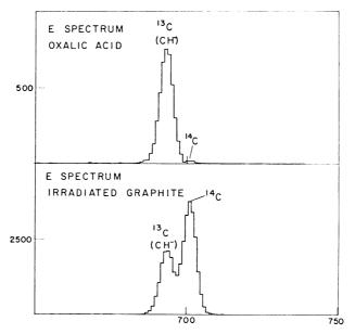
Fig 4. Spectra from irradiated graphite and NBS oxalic acid samples showing the vicinity of the E peak in more detail. Velocity filter is on and a  $2mg \text{ cm}^{-2}$  mylar foil is in front of the E counter. The <sup>13</sup>C background peak arises from charge exchange in the magnet box as described in the text.
