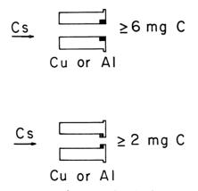
Fig 6. Two sputter source sample geometries. At the top, carbon is sputtered by reflected Cs ions as well as those passing through the central hole. Numbers are the smallest sample sizes used to the present in each geometry.
