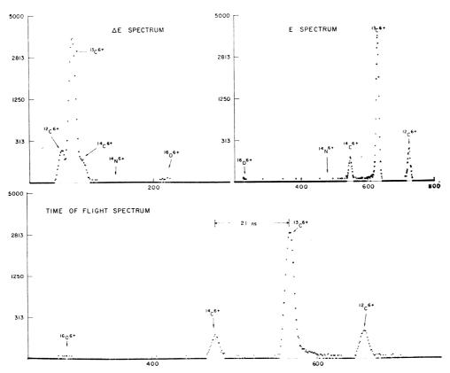
Fig 2. Typical  $\Delta E$ , residual energy, E, and time-of-flight spectra from a <sup>14</sup>C experiment at the Q3D. Spectra are plotted on a square root ordinate scale.
