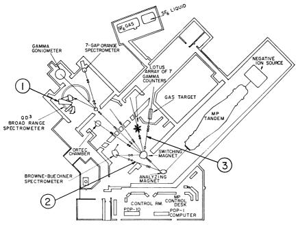
Fig 1. Layout of the Chalk River MP Tandem Complex with locations of <sup>14</sup>C dating experiments indicated by number as follows: 1) Q3D spectrometer; 2) 70° line from the analyzing magnet; 3) 56° line from the switching magnet. Approximate distances to the three positions are 31, 9 and 15m, respectively.
