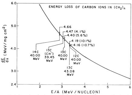
Fig 5. Energy loss of carbon ions in hydrocarbons vs specific energy.  $\Delta E$  values for various background groups are shown. The numbers in parentheses are the percent difference in  $\Delta E$  relative to 40MeV <sup>14</sup>C.
