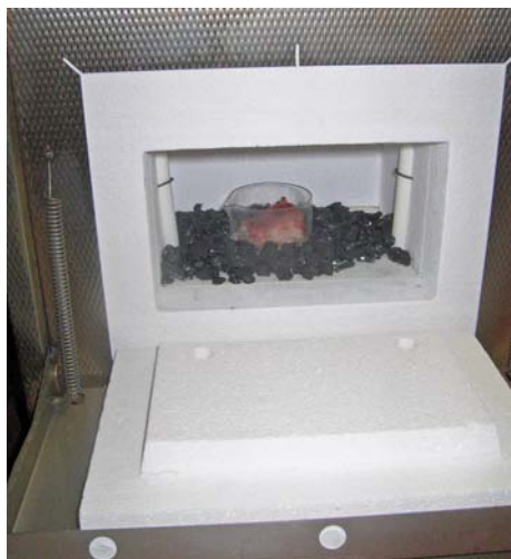
Figure 2 Electric furnace filled with coal and a quartz crucible containing the animal bone.
