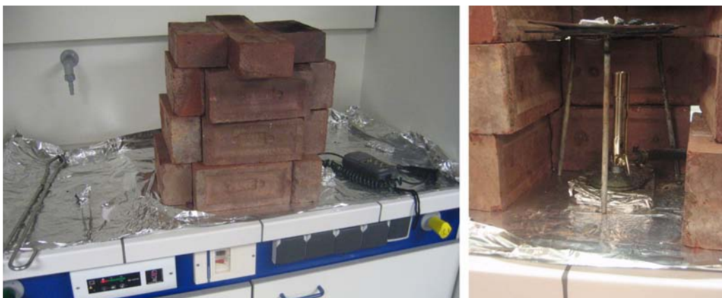
Figure 1 Brick oven used in test 1 (left: general view, right: the bunsen and the calcined bones).
