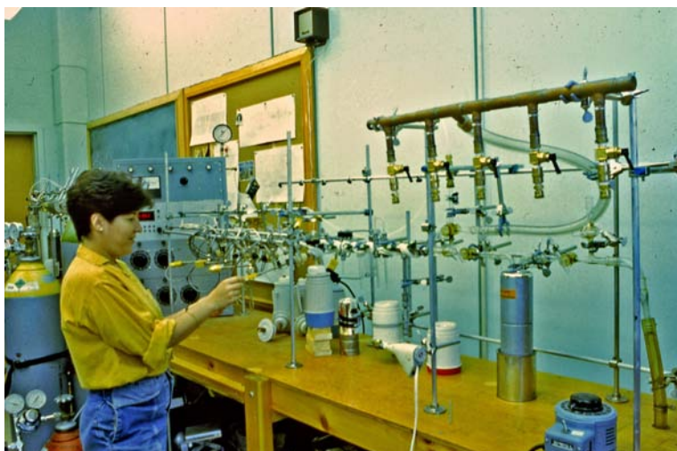
Figure 7 Graduate student H Roman operating John Vogel's "graphitizer" for preparing carbon samples, the progenitor of most (all?) of its kind.
