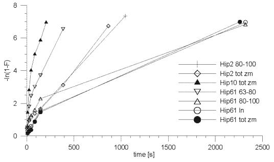
Figure 2 Leaching reaction of different samples from the NW Church in Hippos. Cumulative CO<sub>2</sub> pressure is represented by  $-\ln(1-F)$ , where  $F = p/p_{tot}$  and plotted versus time, and  $p_{tot}$  is the pressure of CO<sub>2</sub> at the end of the reaction.
