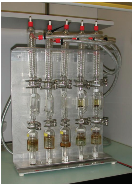
Figure 1 Soxhlet apparatus at the ETH laboratory is used for treatment of textiles prior to ^{14}\text{C} dating. Solvents are boiled below the samples (yellow liquid) and condensed pure liquid refills the sample container (in the middle).
