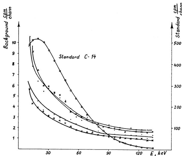
Fig 2. Energy spectra of  $^{14}\text{C}$  and background with the active guard switched on (lower curves) and switched off (upper curves). ○ —  $^{14}\text{C}$ , × — background with quartz vial, ● — background with aluminum vial.
