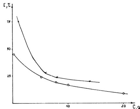
Fig 1. Active guard efficiency in reducing background with different amounts of scintillation cocktail.  $\times$  — plastic scintillator,  $\circ$  — Geiger-Mueller counters.
