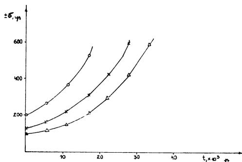
Fig 5. Statistical error with different amounts of scintillation cocktails (24hr measuring cycle). ● — 0.1g C, × — 0.3gC, ▲ — 0.6g C.
