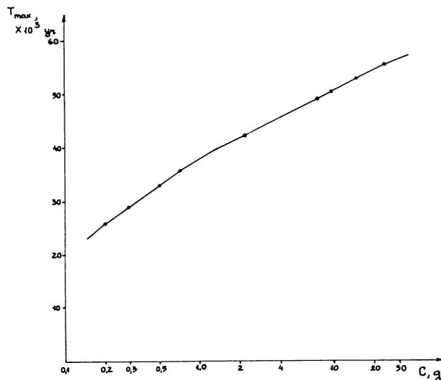
Fig 4. Maximum ages determinable with different amounts of scintillation cocktail (48hr,  $3\sigma$ ).
