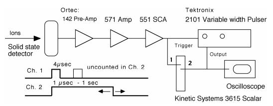
Figure 3 Apparatus for determining the dependence of scalar live time on the ion arrival time distribution
