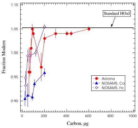
Figure 2 Fraction modern measured on small HOxI standards after normalizing to standard-sized HOxI. Results are shown for Arizona and for two different graphite catalysts used at NOSAMS. In practice, rather than try to derive an equation for the behavior of the standards, most laboratories run a large number of small standards with their small samples.
