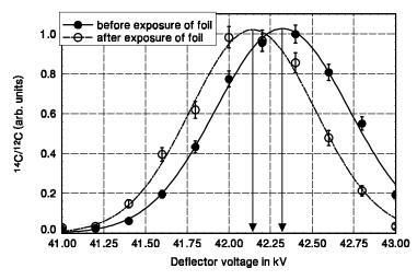
Figure 5 Scans with the  $180^{\circ}$  deflector (located in the terminal of the accelerator) taken before and after a few hours of foil exposure. The solid and dashed lines are representing gaussian fits. The terminal voltage was set to 750 kV and the resulting shift in particle energy between both measurements is calculated to be 3.1 keV.
