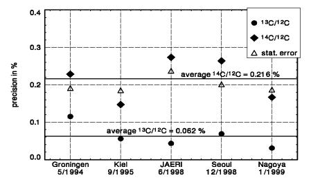
Figure 2 Results from the acceptance tests of the five HVEE <sup>14</sup>C-AMS systems. The data show the average precision from two succeeding days for  ${}^{14}C/{}^{12}C$  and  ${}^{13}C/{}^{12}C$ , as well as the averaged uncertainty from the counting statistics. Six modern samples were measured on each day.
