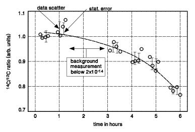
Figure 4 <sup>14</sup>C/<sup>12</sup>C precision measurements with the biomedical <sup>14</sup>C IRMS. Four samples have been used in six runs. Between runs 2 and 3, a background sample (commercial graphite) has been measured. The dashed line is a weighed spline fit through the averages of each run and is meant to guide the eye.
