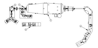
Figure 6 Layout of the new AMS system, based on a 5 MV Tandetron  $\bigcirc$ , with a simultaneous injector for high precision <sup>14</sup>C-AMS  $\bigcirc$ , a sequential injection system for multi-element AMS with an optional ion source  $\bigcirc$ , the high-energy section B and the computer control D.
