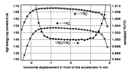
Figure 1 Horizontal steerer scan of  ${}^{13}C$  and  ${}^{12}C$  currents measured in the high energy Faraday cups of the 3 MV  ${}^{14}C$ -AMS machine
