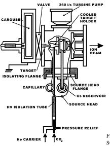
Figure 3 Schematic layout of the negative ion source SO110 for solid as well as and CO<sub>2</sub> samples
