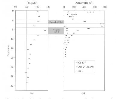
Figure 2 Radionuclide analyses of a composite peat sequence from the west coast site (Louisburgh) showing (a) <sup>14</sup>C and (b) <sup>7</sup>Be, <sup>137</sup>Cs and <sup>241</sup>Am profiles. Strata approximating to 1986 (Chernobyl event) and 1964 (weapons fallout peak) are also indicated on the diagram. Note, <sup>241</sup>Am values are scaled up by a factor of 10 for ease of display. Error bars represent  $\pm$  1 S.D.
