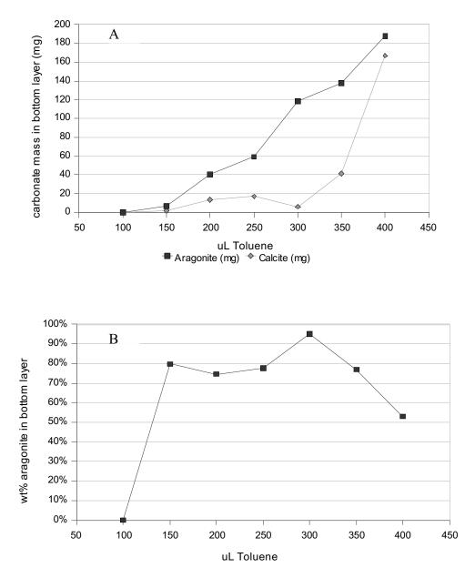
Figure 2 (A) Graphical results of the CarDS optimization showing mass of calcite and aragonite in the bottom layer of each separation, with the volume of toluene added to 4.0 mL of bromoform. (B) The percentage of aragonite in the bottom fraction with respect to the volume of toluene added. Clearly, the optimum separation is achieved with 300  $\mu$ L of toluene, giving a solvent density of 2.75 g/cm<sup>3</sup>. Details of the experiment can be found in the text.
