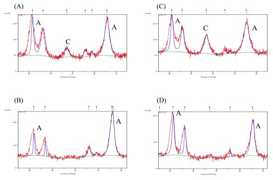
Figure 3 (A) and (B) show the top and bottom layers, respectively, from the CarDS separation of a shell from Taperinha; (C) and (D) the same for a shell from Viking Bank. Characteristic peaks are marked with A for aragonite and C for calcite. Clearly, the bottom layers contain significantly less calcite than the top layers, demonstrating the effectiveness of CarDS.
