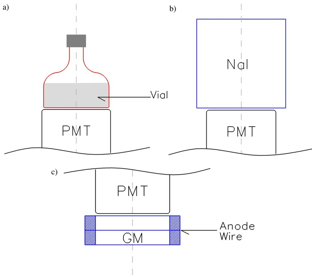
Figure 1 Detectors used in the study: a) 3-mL vial with PMT; b) NaI with PMT; c) low-level Geiger counter for measuring beta emission from the face of the PMT.
