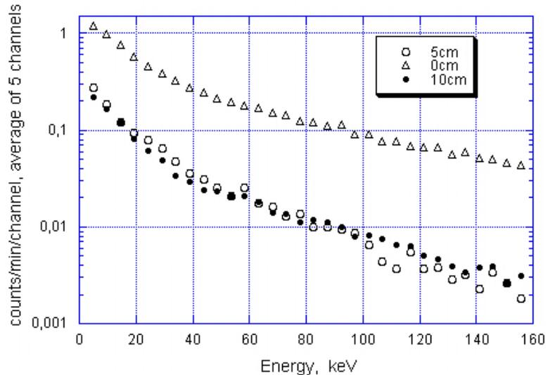
Figure 5 The LS background spectra in the underground counting room, unshielded and inside 5- and 10-cm-thick lead shields.
