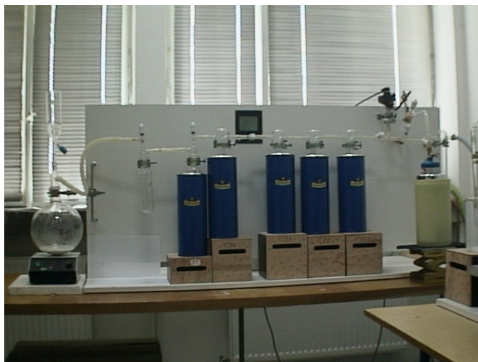
Figure 2 Line for \text{BaCO}_3 acidification and \text{CO}_2 purification
