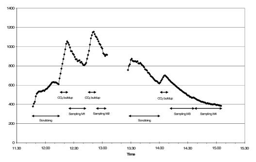
Figure 3 Temporal changes in  $CO_2$  concentration during scrubbing, build-up, and sampling of  $CO_2$  during the testing of the method.
