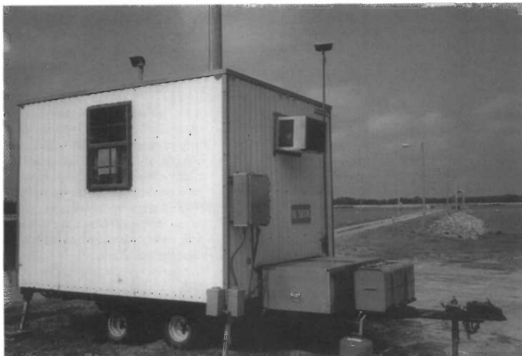
Fig. 5. Trailer housing for FDTAS field unit
