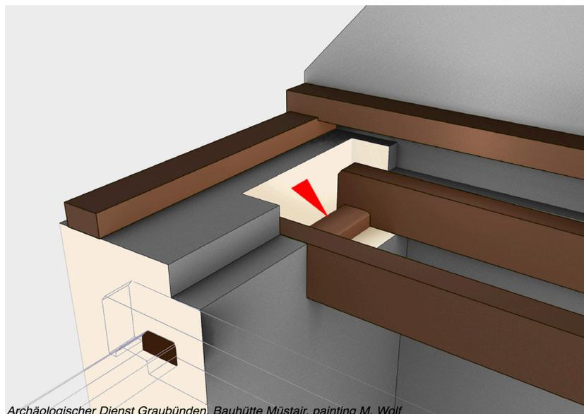
Figure 2 The drawing shows the location of the dated wall lath (M06/24'255) in the wooden beam ceiling of the Holy Cross chapel.
