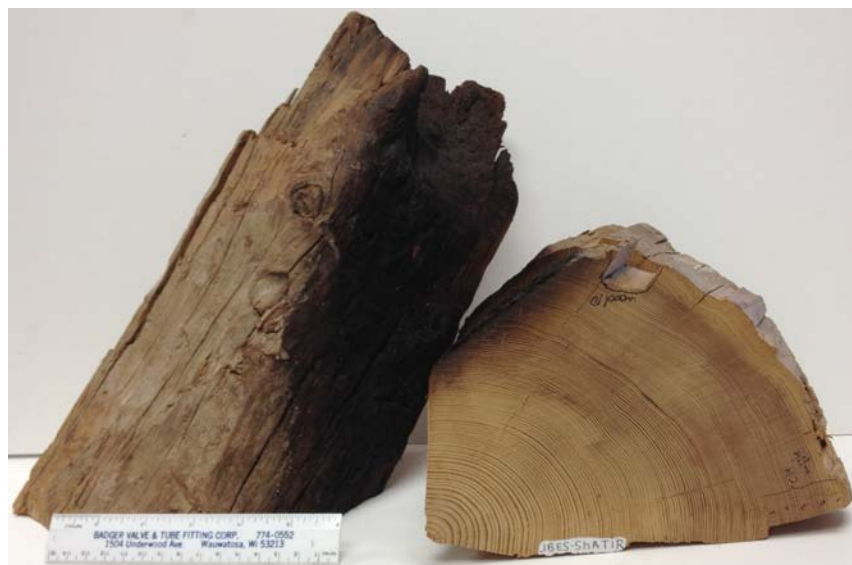
Figure 1 Photo of wood specimen #1 subsampled for 14 C dating. The charred end is the result of a fire that occurred in the Bes-Shatyr #3 tomb around the time of construction.
