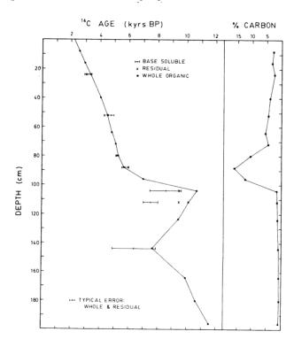
Fig. 2. The <sup>14</sup>C age vs depth for whole organic carbon, base-soluble fraction, and residual sediment from core 1443 from the Black Sea. The organic carbon content of the core is also shown, indicating the carbon-rich, sapropelic layer. Humic material from the sapropel diffused into the older carbon sediment below 100 cm.
