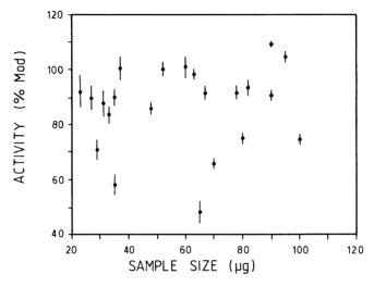
Fig 1. Final  $^{14}$ C concentrations as a function of carbon sample size for 22 samples < 100  $\mu$ g from a study of the ecosystem around a marine oil seep.  $^{14}$ C concentrations were measured to a precision of 1–2%. Final precisions were 3–8% after size-dependent background subtraction.
