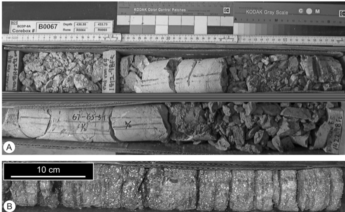
Fig. 14. Fracturing (a) and disking (b) in core LB-08A. a) Rows one and five of box B0067 comprise intervals with rubble only (“fracturing of type 5” in the profile of Fig. 3). Note the sharp boundary of apparently coherent material that breaks to pieces if even only slight pressure is applied. The fracturing is due to impact-induced weakening of the target rocks. b) Meta-graywackes in row three of box B0011 display severe disking in individual disks with a thickness ranging from 1 to ~5 cm. This type of disintegration is assumed to be caused by drilling.
