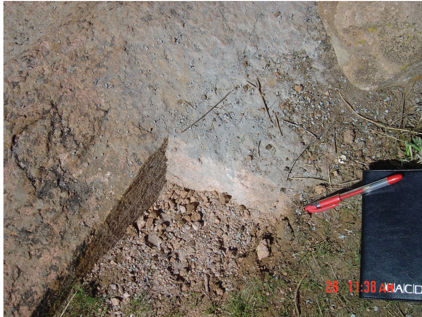
Fig. 2. The shocked and broken granite plate on which stone II impacted. Note the gray dust derived from the stone upon impact.
