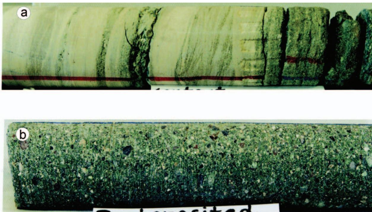
Fig. 2. Two core samples of unit 1: a) the transition of laminated Tertiary limestone interlaminated with thin suevitic material and laminated, redeposited suevite below; b) clast-size sorted suevite. Cores have a diameter of 64 mm.
