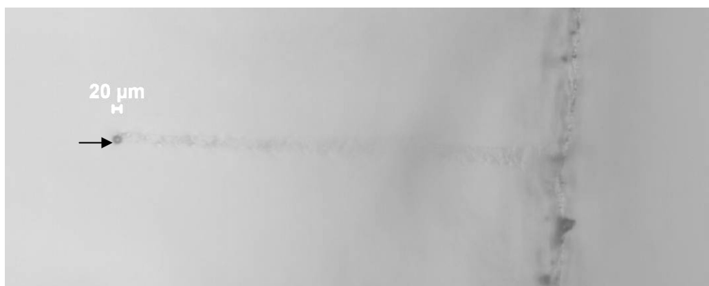
Fig. 5. Example track in aerogel for impact of 20 \mu\text{m} polystyrene microparticles coated with 20 nm polypyrrole at an impact speed of 1.07 \text{km s}^{-1} (the impact was from the right). A whole track is shown, with a total length of 1088 \mu\text{m} . The front face of the aerogel appears as a near-vertical line near the right-hand side of the image. The track is the faint, tapering cylinder across the middle of the image and the captured particle (marked with an arrow) is in the left of the image at the end of the track.
