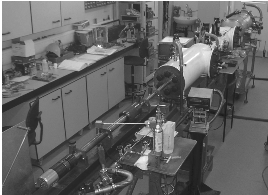
Fig. 1. The University of Kent two-stage light gas gun (LGG). The gun is 5 m in length and in this image fires from bottom left to top right.
