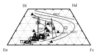
Fig. 9. Pyroxene quadrilateral compositions for SaU 300 superimposed on the two-pyroxene thermometer of Lindsley and Anderson (1983). Open triangles = matrix px; closed triangles = px fragment; open squares = lithic clasts. Pyroxenes both follow and lie between the 1000 °C and 1200 °C isotherms. Matrix compositions mostly lie along the 1100 °C isotherm.
