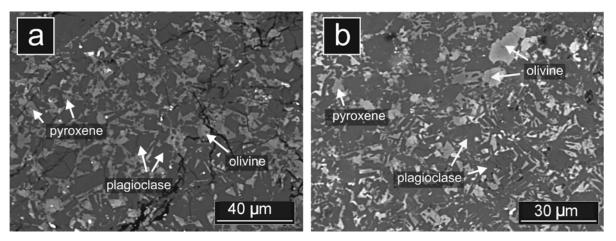
Fig. 1. BSE images of the matrix of SaU 300. a) Three main phases are plagioclase, pyroxene, and olivine. b) Olivine shows reaction texture (anhedral to subhedral shapes). White phases are FeNi metal.
