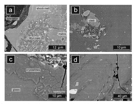
Fig. 7. BSE images of melt textures in SaU 300. a) Melt margin showing gradational boundary between schlieren-rich melt containing abundant spheres/blebs of Fe oxides and a lithic clast. b) A relatively cold clast entrained within the melt. c) Quench margin of the shock melt in contact with host rock. d) Schlieren-rich melt.
