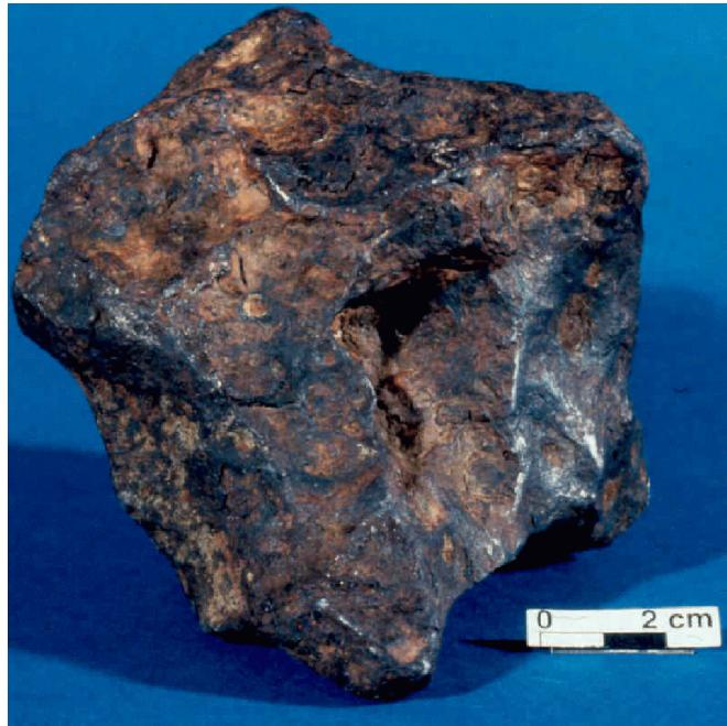
Fig. 1. The Toronto IAB iron,  $\sim 10 \times 8 \times 7.5$  cm in size, mass 2.715 kg.
