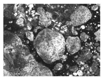
Fig. 9. Liquid immiscibility between silicate-rich glass and carbonates (sample NMNH 113029-15). Width of view is 2 mm.
