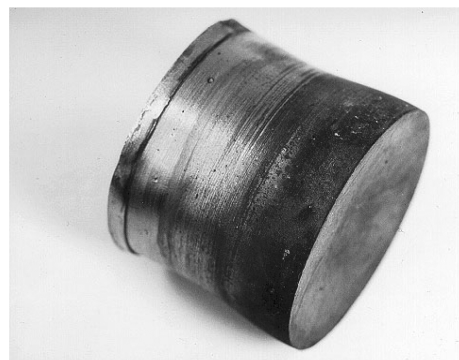
Fig. 2. a) Driver plate and steel blocks after deformation; b) Armco-iron container after deformation at 45 GPa.
