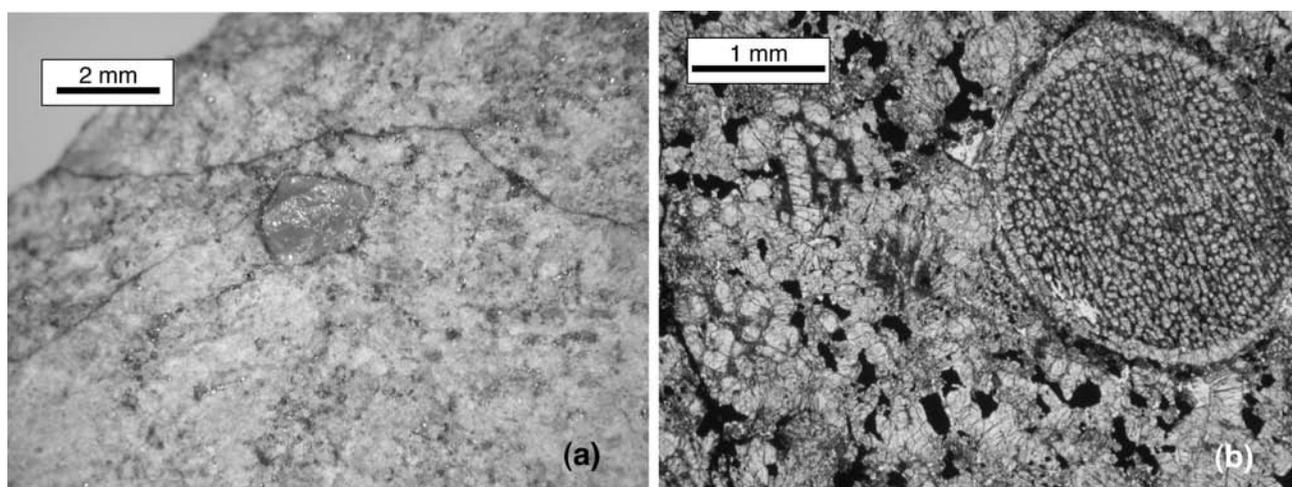
Fig. 3. a) Stereomicrophotograph of a freshly broken surface of Beni M'hira showing a 2 mm-sized glass inclusion set in a homogeneous crystalline matrix crosscut by dark shock veinlets; b) transmitted light photomicrograph of Beni M'hira showing a mm-sized, highly recrystallized, barred olivine chondrule relic set in a granoblastic matrix.
