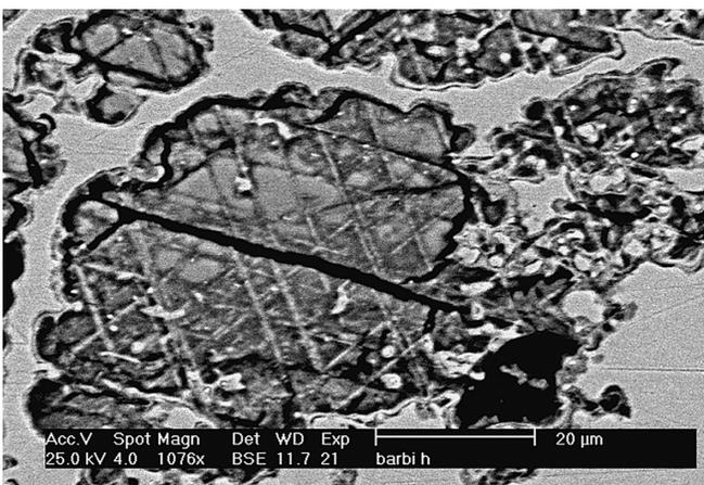
Fig. 4. Detail of dark region showing three regular sets of intersecting lines. Lines can be either darker or lighter than the host and likely mimic the cleavage structure of the original metal. Lighter lines might represent exolved lamellae of distinct composition.
