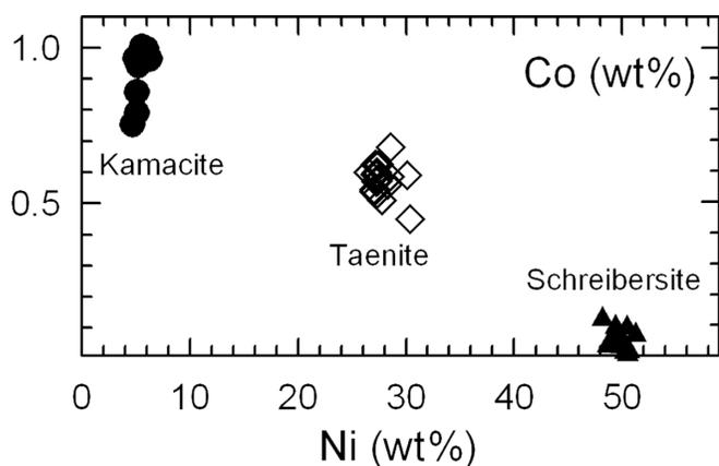
Fig. 6. Variation diagram of Co versus Ni in the main mineral phases of the Barbianello iron meteorite shows a good negative correlation.
