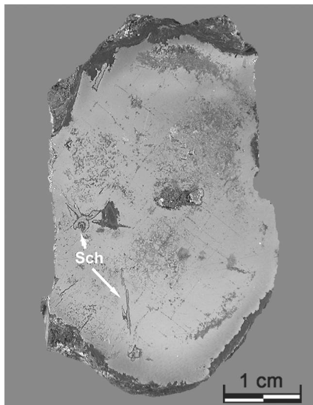
Fig. 1. Polished surface of a chip of the Barbianello iron meteorite. Alteration on the newly polished surface, corresponding to the dark regions, is evident. White arrows indicate schreibersite crystals (photograph by Stefano Castelli [2001]).
