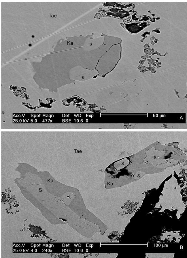
Fig. 3. Backscattered electron image of the Barbianello iron meteorite. Kamacite (Ka) is found in isolated irregular, subrounded pods or around grains and shafts of early-crystallized schreibersite (S). Taenite (Tae) represent the main component. The irregular dark areas surrounding black zones (holes and fractures) represent domains of alteration.
