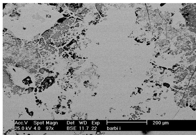
Fig. 2. Backscattered electron image of the Barbianello iron meteorite with light and dark regions arranged in a sort of geometrical pattern. Kamacite (Ka) is only present within the light regions.
