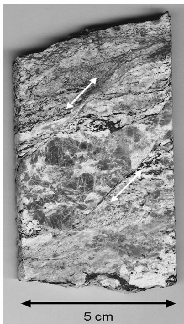
Fig. 2. Crystalline basement displaying brittle fractures from the W-1 core (sample #W-15 from 193.7 m). The arrows point to the area of possible shear deformation.
