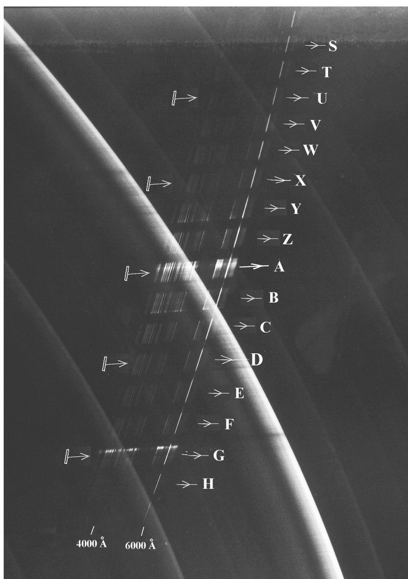
Fig. 1. The Andromedid spectrum (AND) analyzed in this work. The spectrum is divided into segments due to the rotating shutter.
